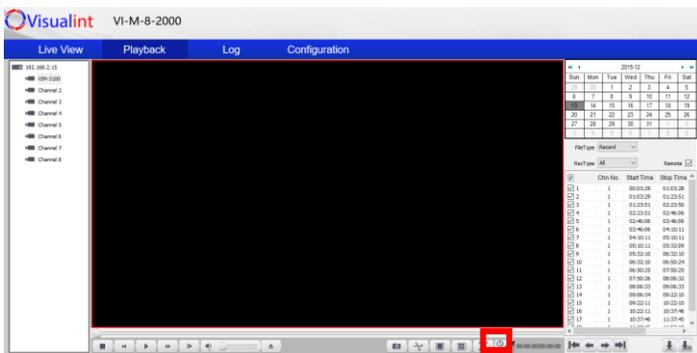
Switch Mode toggles to the export video interface. Note the File Type & RecType drop down. Use these drop downs to filter the saved recordings. Recordings are sorted by channel number and segregated accordingly.
