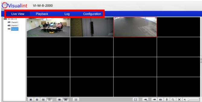
The upper navigation bar allows access to Playback, Alarm Logs and NVR Configuration.
