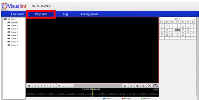
Playback allows access to recorded video. Select your channel, date from the calendar and use the lower timeline to select the desired time of day.
